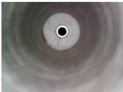
LC9 - Residues detected after 14 cm of insertion.
