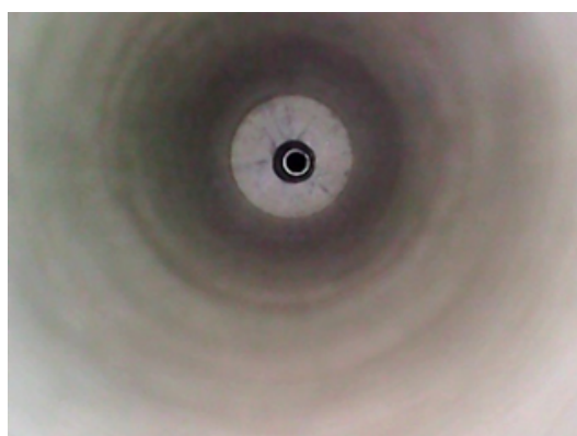
LC6 - Grooves detected after 9 cm of insertion.
